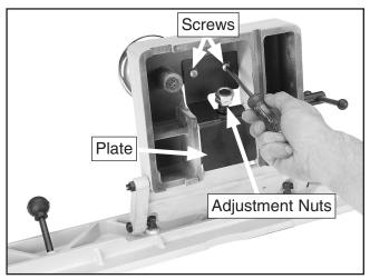
**Figure 61**. Removing plate to access inward fence stop.
